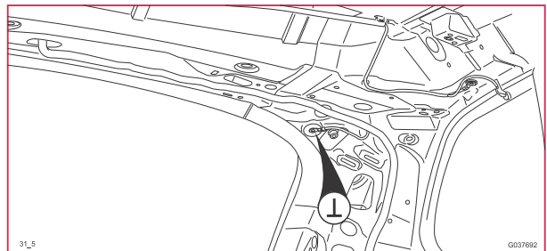
31/5 Ground connection, rear edge roof
